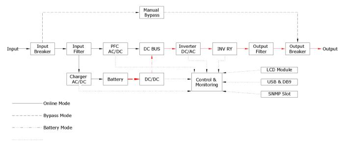
Figure 4 Single Line Drawing - Battery Operation
