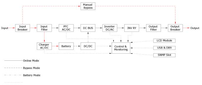
Figure 3 Single Line Drawing - Static Bypass Operation
